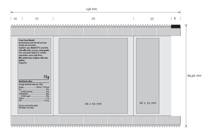
Sealed seam, 10 mm Overlapping seam, white or transparent Print area for full surface print
